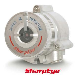
The new 40/40R Single IR Flame Detector detects bydrocarbon-based fuel and gas fires using advanced flame analysis tools. The detector provides early warning of flaming fires working at 4.5 um for maximum sensitivity, and immunity to false alarms from IR sources such as sunlight and IR projectors.
