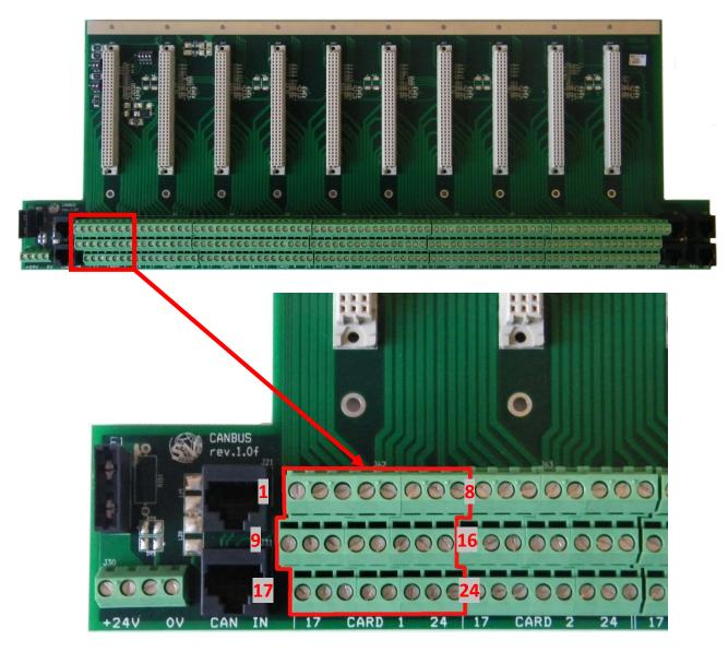
Terminals are power limited to avoid danger in the event of short circuit. Technical specifications of the terminal strip are summarized as follows:
