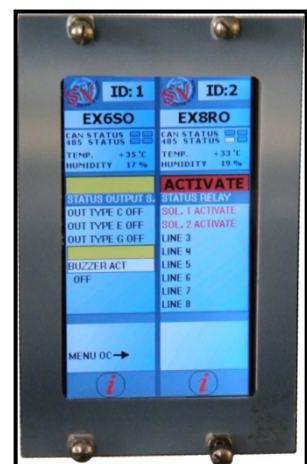
Touch-screen displays of I/O modules
